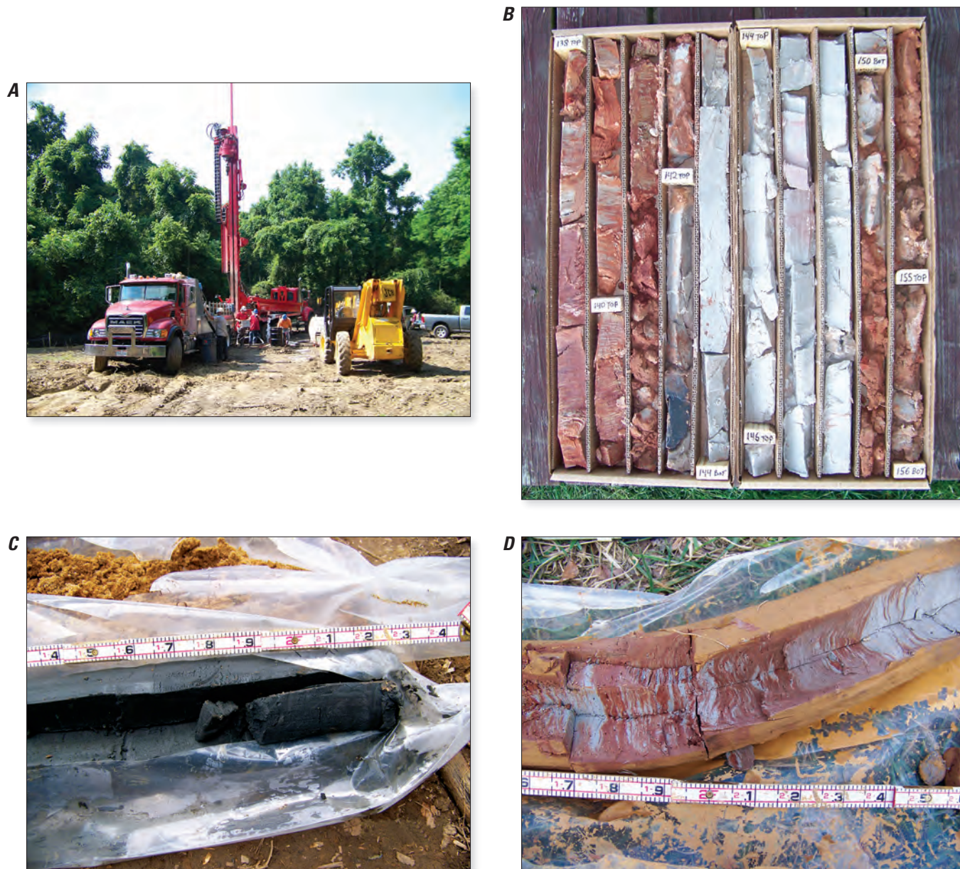
Figure 6. Photographs showing (A) rotonic drilling, (B) recovered core, (C) core from Merchantville confining unit, and (D) core from upper Potomac confining unit. [Photographs by U.S. Geological Survey.]
