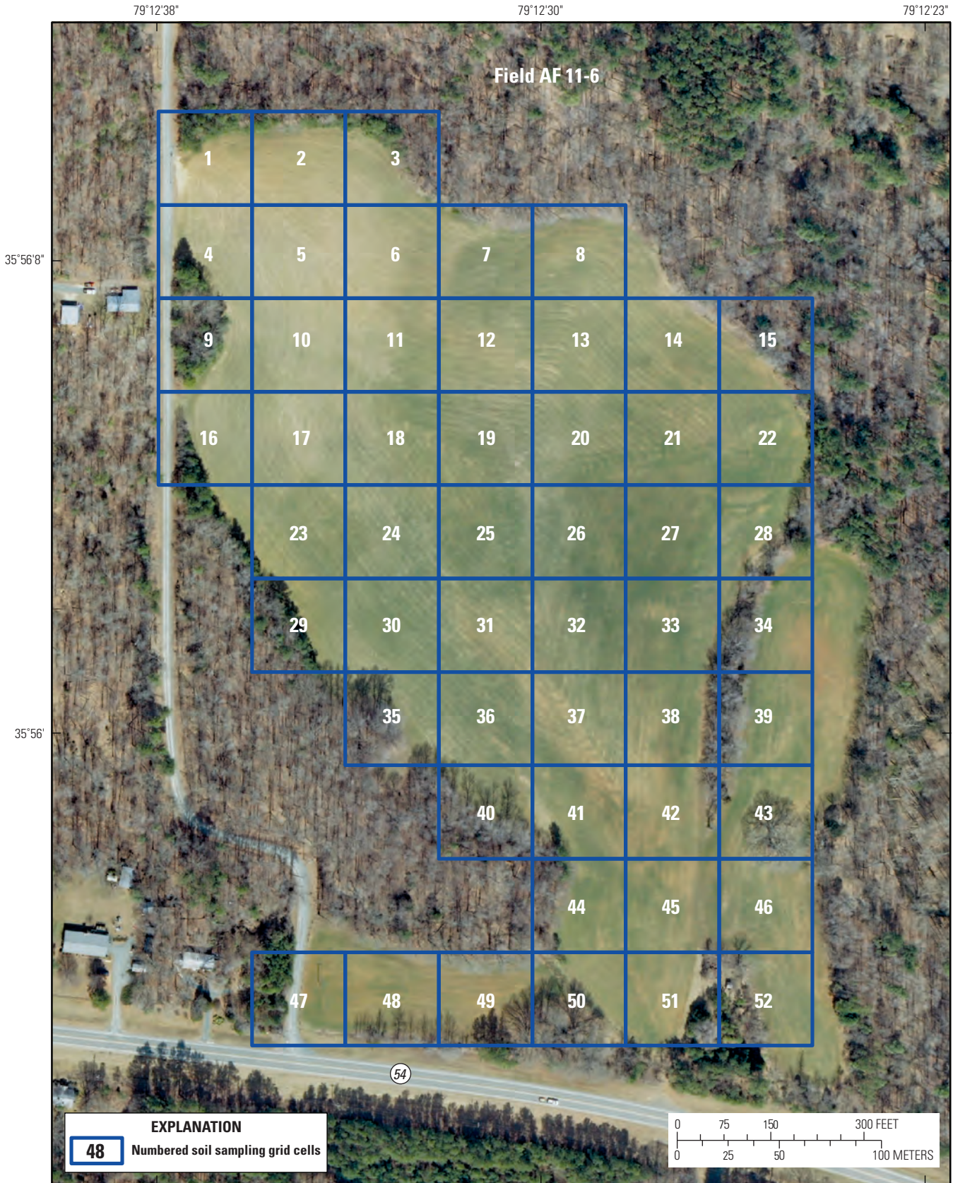
Figure 4. Example of the soil sampling grid at biosolids land-application field AF 11-6 in the Collins Creek watershed in Orange County, North Carolina.
