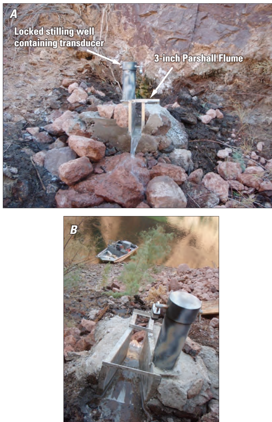
Figure 5. Monitoring site showing flume and stilling well, looking (A) toward seep, and (B) toward the Colorado River at Arizona Hot Spot in Black Canyon, Lake Mead National Recreation Area, Nevada and Arizona. Photographs taken by Jon Wilson, U.S. Geological Survey, 2008.
