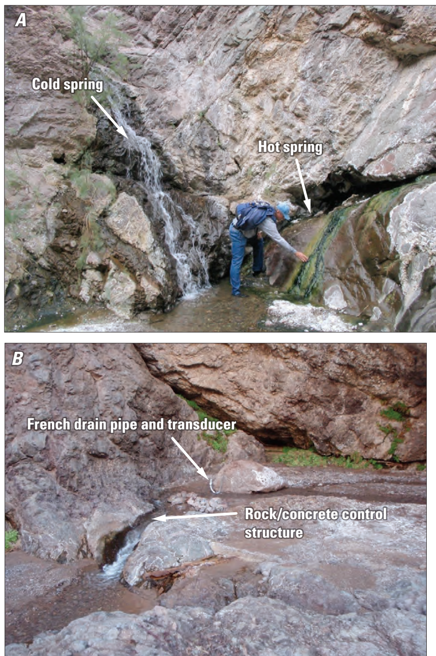
Figure 7. Monitoring site showing (A) hot and cold springs that contribute to the main channel upstream of monitoring site; and (B) French-drain pipe, transducer, and rock/concrete control at Boy Scout Canyon in Black Canyon, Lake Mead National Recreation Area, Nevada and Arizona. Photographs taken by Jon Wilson, U.S. Geological Survey, 2009.
