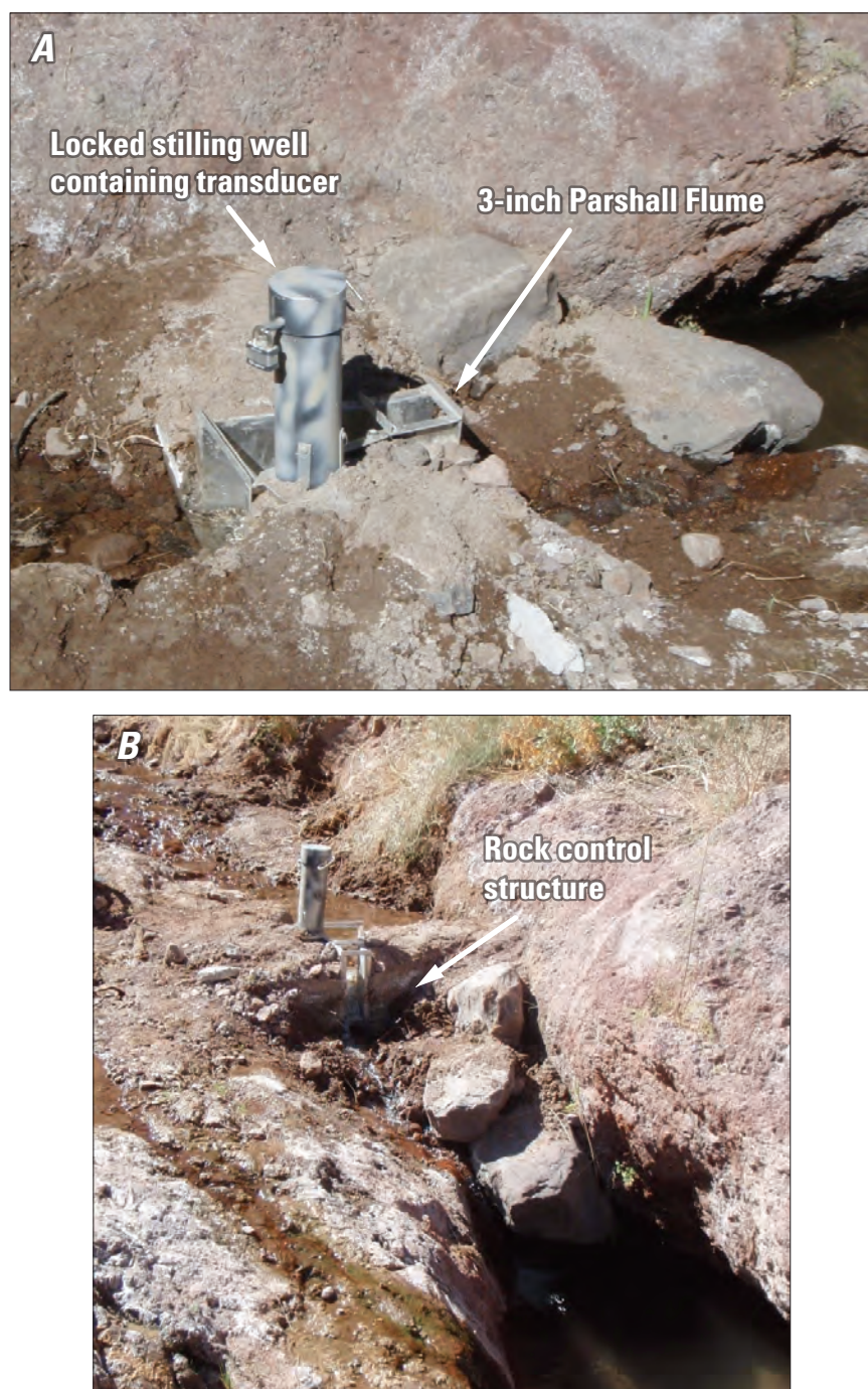
Figure 8. Monitoring site showing (A) flume and stilling well installed at stream, and (B) rock/concrete control downstream of monitoring site at Bighorn Sheep Spring in Black Canyon, Lake Mead National Recreation Area, Nevada and Arizona. Photograph taken by Jon Wilson, U.S. Geological Survey, 2009.
