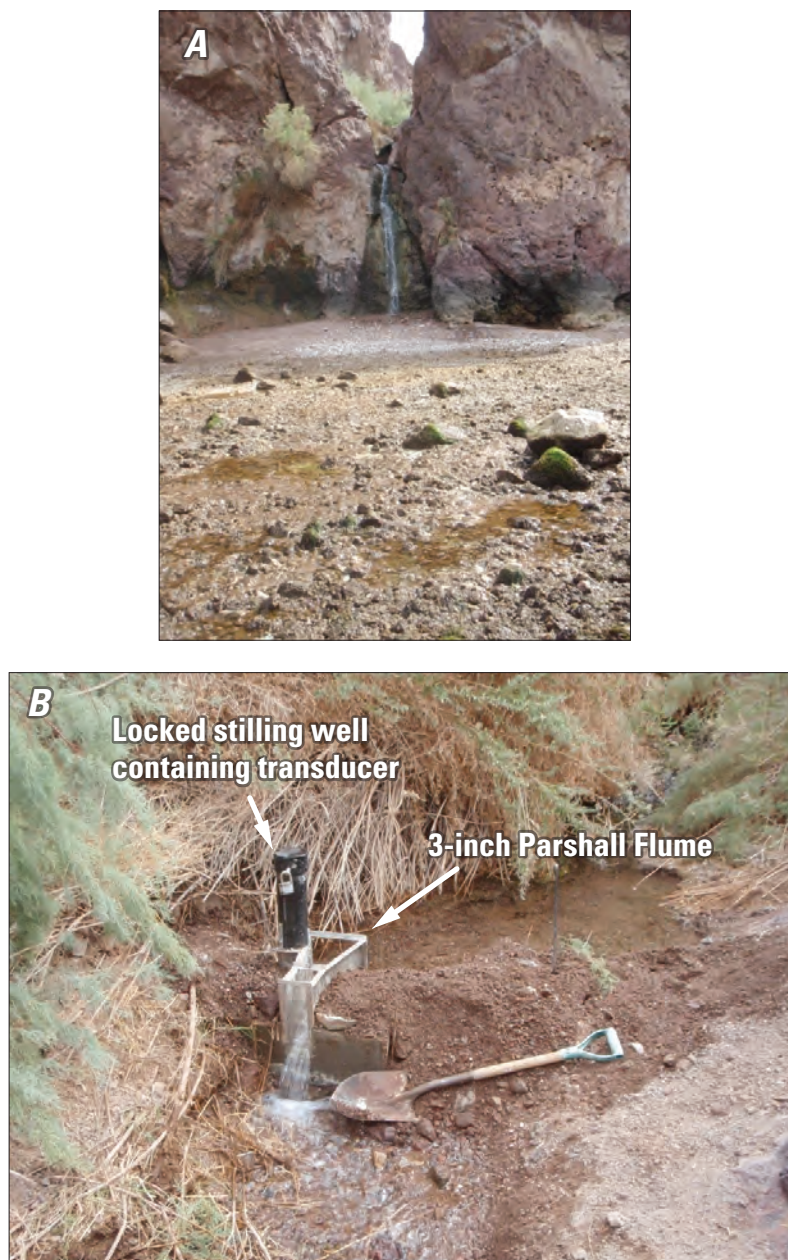
Figure 6. Monitoring site showing (A) waterfall immediately downstream of monitoring site, and (B) monitoring site with flume and stilling well installed at stream at Palm Tree Spring in Black Canyon, Lake Mead National Recreation Area, Nevada and Arizona. Photographs taken by Jon Wilson, U.S. Geological Survey, 2008.
