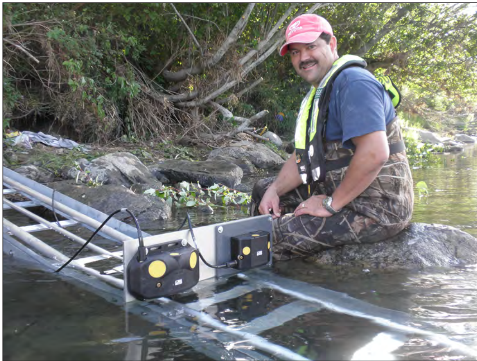
Figure 3. U.S. Geological Survey scientist installing and servicing 1.5-megahertz (MHz; left) and 3.0-MHz (right) SonTek®/Xylem acoustic Doppler velocity meters attached to an aluminum slide track mount at the Crossport site (USGS 12308500), Kootenai River, Idaho. (Photograph by Molly Wood, U.S. Geological Survey, August 30, 2010.)
