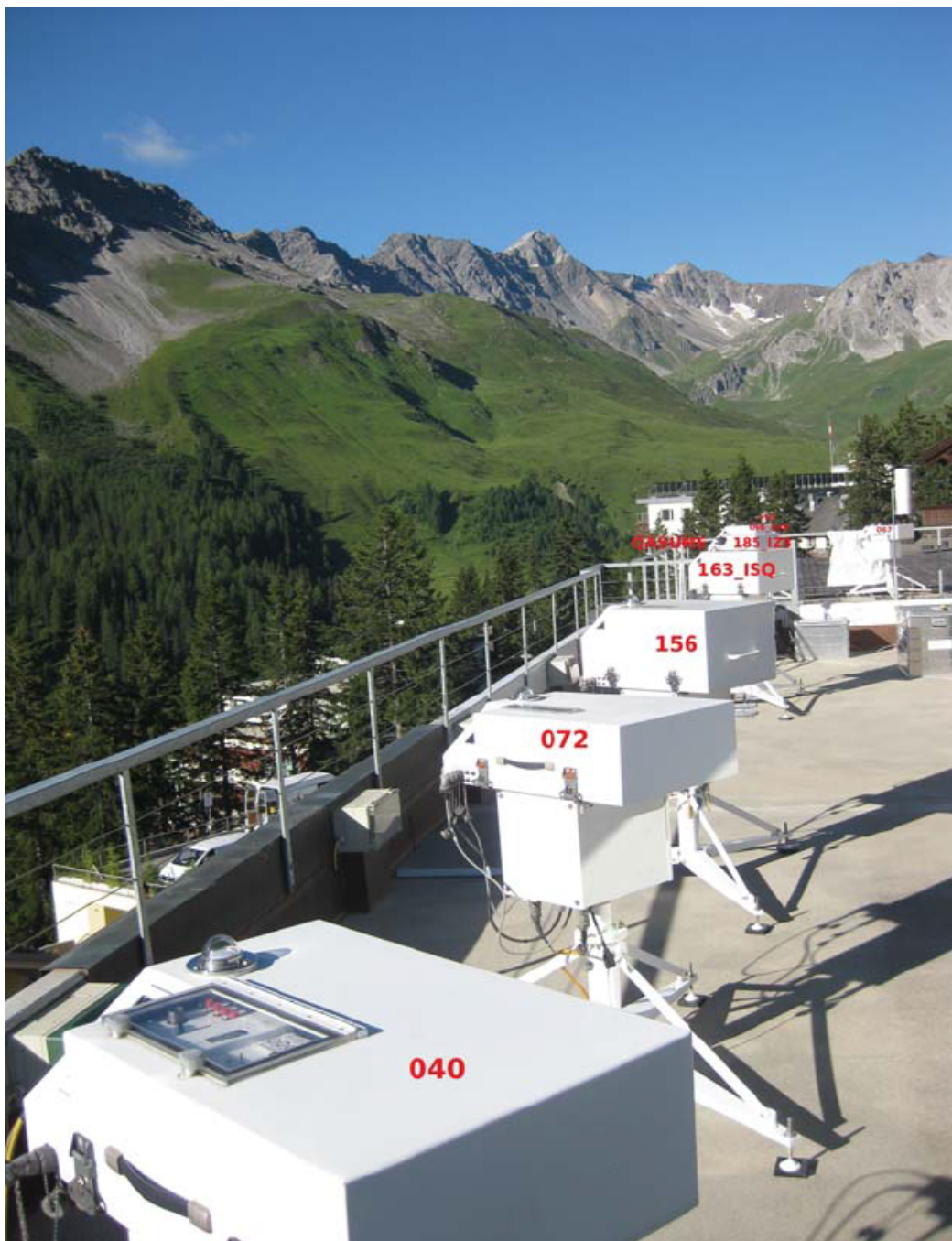
Figure 5. Overview of the measurement platform at LKO Arosa with the participating Brewer spectrophotometers
