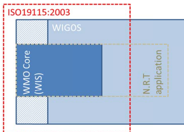
Figure 4. Schematic of the relationship of WIS and WIGOS metadata and the scope of the ISO19115 standard. The WMO Core is a profile of ISO19115. WIGOS metadata exceed the scope of ISO19115 standard. A possible profile (subset) of WIGOS metadata elements for some specific near-real-time application is also shown.
