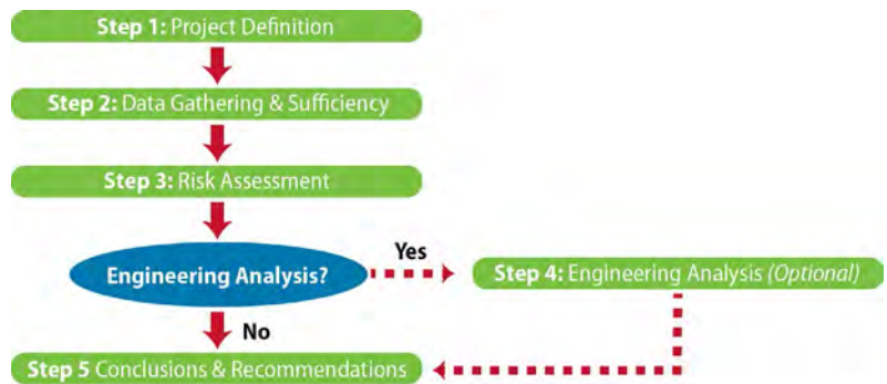
FIGURE 2: An overview of the PIEVC five step process to analyze the engineering vulnerability of an individual infrastructure to current and future climate (Source: PIEVC, 2007).
