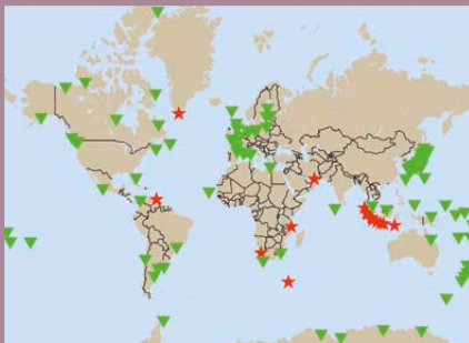
▲ Network of GPS stations at tide gauges (green triangle: TIGA observing stations; red star: stations in the test phase)
