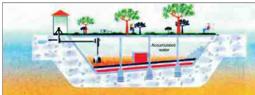
Figure 5.26: Detention pond with pumping
