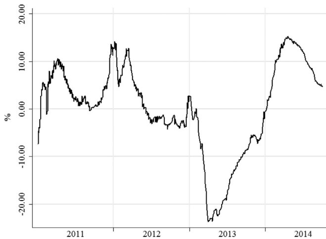
Fig. 5. Difference between current filling grade and the average seasonal filling grade of the past 3 years for the countries Belgium, France, Germany, Italy, the Netherlands and the United Kingdom. Source: gas storage: GIE, CUGS and GTS; HDD: ECA&D; own calculations.
